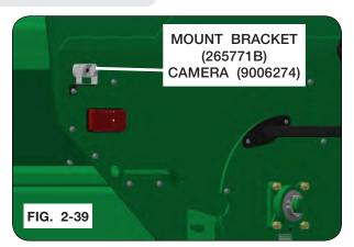
NOTE: If more cable length is needed, connect 16' camera cable (9007174).
