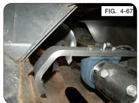
21. Extend a string tightly from front to rear to check horizontal auger alignment. Measure the string to the auger tube either in front or behind the hanger bearing. If this dimension is 1/8" greater than the measurement taken in the front and rear, shims (8GA - 286419B or 12GA - 286424B) are required on top of the center hanger bearing. Ideally the center measurement should be equal to or 1/8" lower than the measurements on the ends of the augers. (Figure 4-68)
